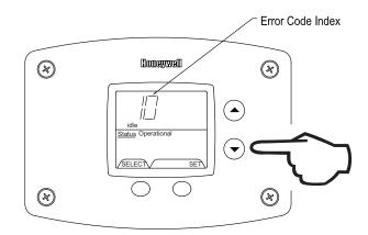
Step 3: Press the "Select" button to view the error code for "code 10". If there is a number displayed, note what the number is. The label next to the water heater display will identify the code number. If no number is displayed with only a "--" in the water heater display, then there has not been an error code for error code index 10.
